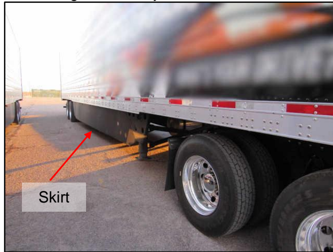
Figure 5: Utility Side Skirt 120A-4
