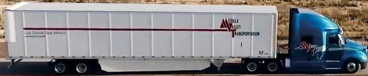
MVTS test results comparing MICHELIN Energy Guard to packages of STEMCO TrailerTail and EcoSkirt solutions showed savings within 1 gallon per 1,000 miles or 1%.
